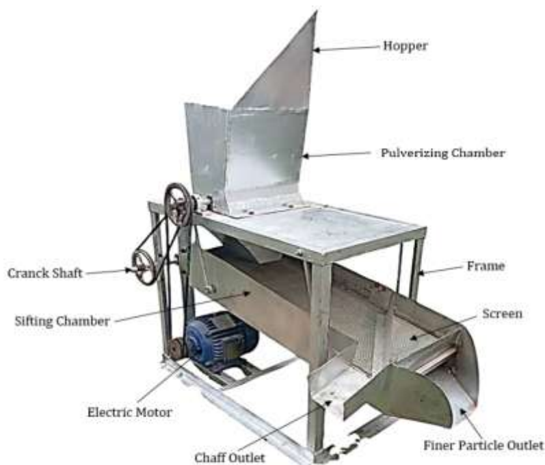
Plate 2: Gari Pulverizing and Sieving Machine
