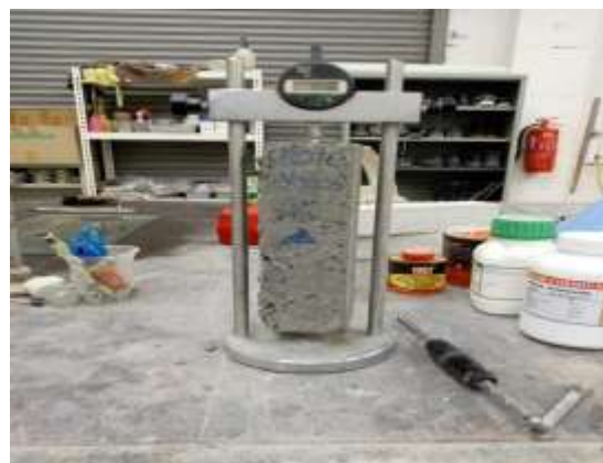
Figure 1: Drying shrinkage Comparator for Top Readings
